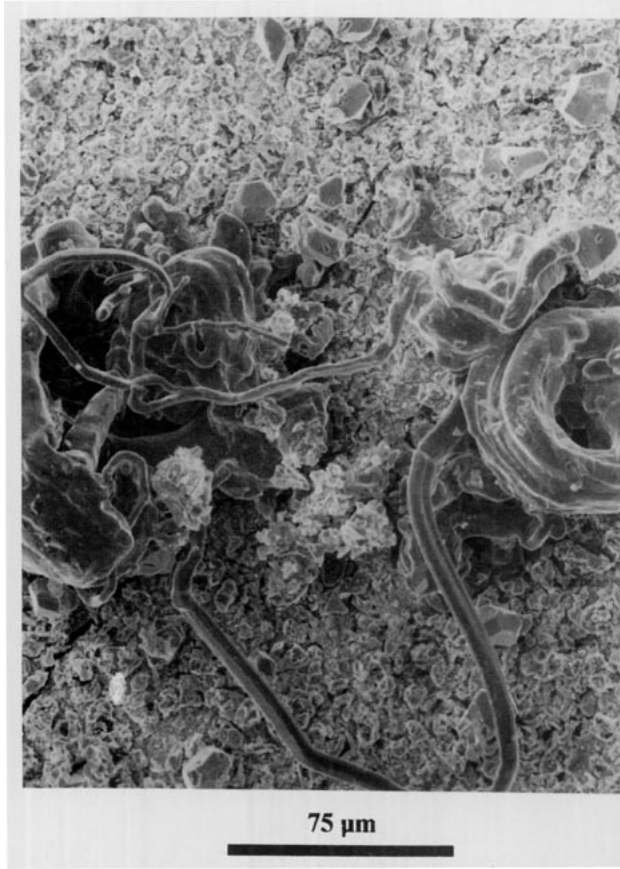
FIG. 3. Whiskers of Cu at the surface of a Y_1Ba_2Cu_3O_{7-x} pellet after sulfurization in the vicinity of the nuclei of Fig. 2.
