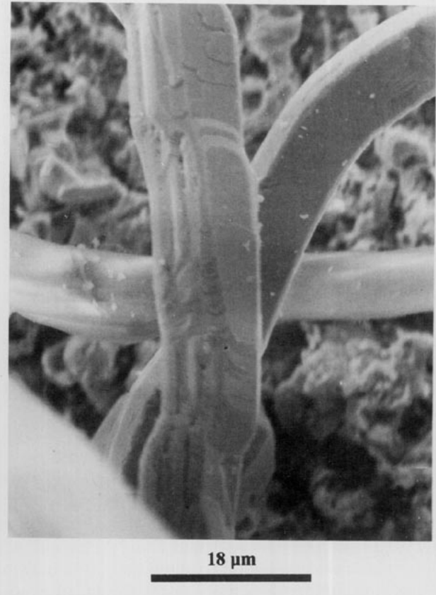
FIG. 4. Whiskers of Cu at the surface of a Y_1Ba_2Cu_3O_{7-x} pellet after sulfurization showing the cross-section uniformity and slip lines.
